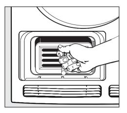
Pull the condenser unit out of its housing by the handle.
